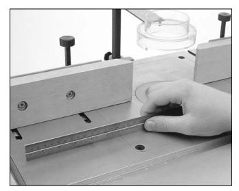
Figure 15. Checking insert for flushness.
